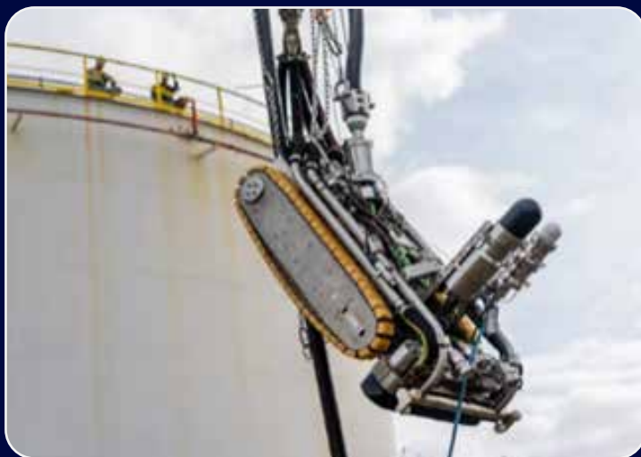
Specialized to perform Tank's on-stream Inspection without Opening
