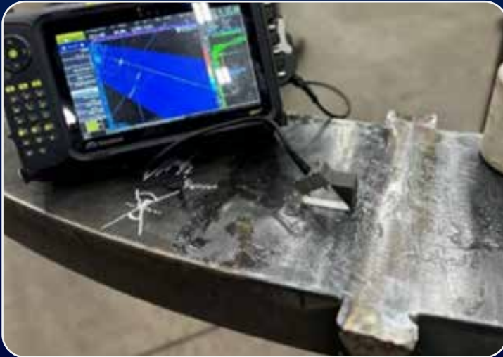
Capability to performed Phased Array Ultrasonic Testing (PAUT)
