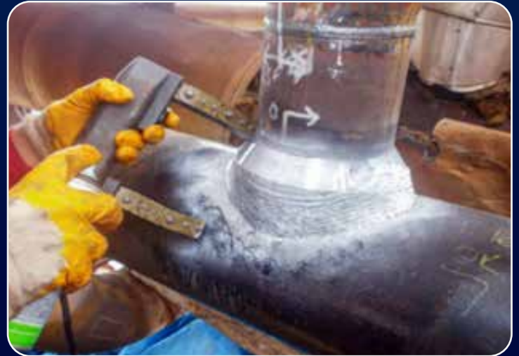
NDT Team to perform the Magnetic particles test ( MT), Dye Penetrant Test (DPT)
